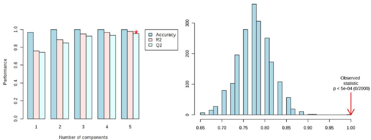
**Figure 6.** Left: Cross-validation showing the 3 performance measures (prediction accuracy,  $R^2$ , and  $Q^2$ ) using different numbers of components. \* indicates the best values of the currently selected measures  $Q^2$  (0.86). Right: the result of permutation test statistics summarized by a histogram ( $P < 5e^{-4}$ ).
